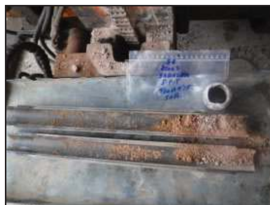
Foto 17: Sondeig S-2, SPT a 9,0 metres.
